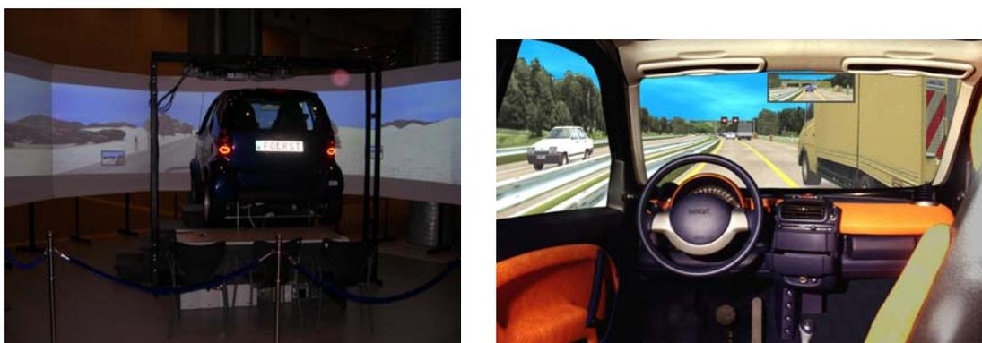
Figure 4 View of the HIT driving simulator (left) and driver's field of view (right)
