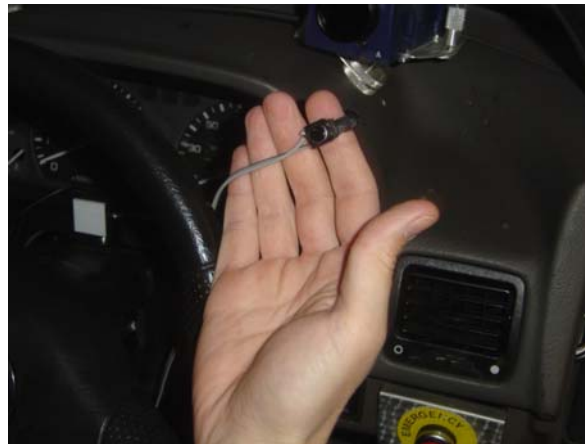
Figure 28 - The response button used for all detection tasks in the Leeds experiment
