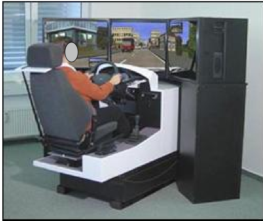
Figure 3. Type B simulator: static or semi-dynamic simple driving simulator.
