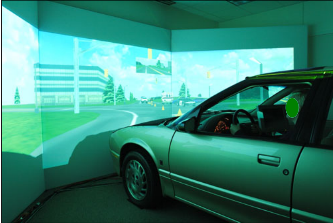
Figure 4. Type C simulator: fixed driving simulator.
