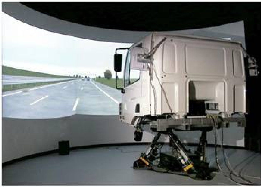
Figure 5. Type D simulator: dynamic driving simulator.
