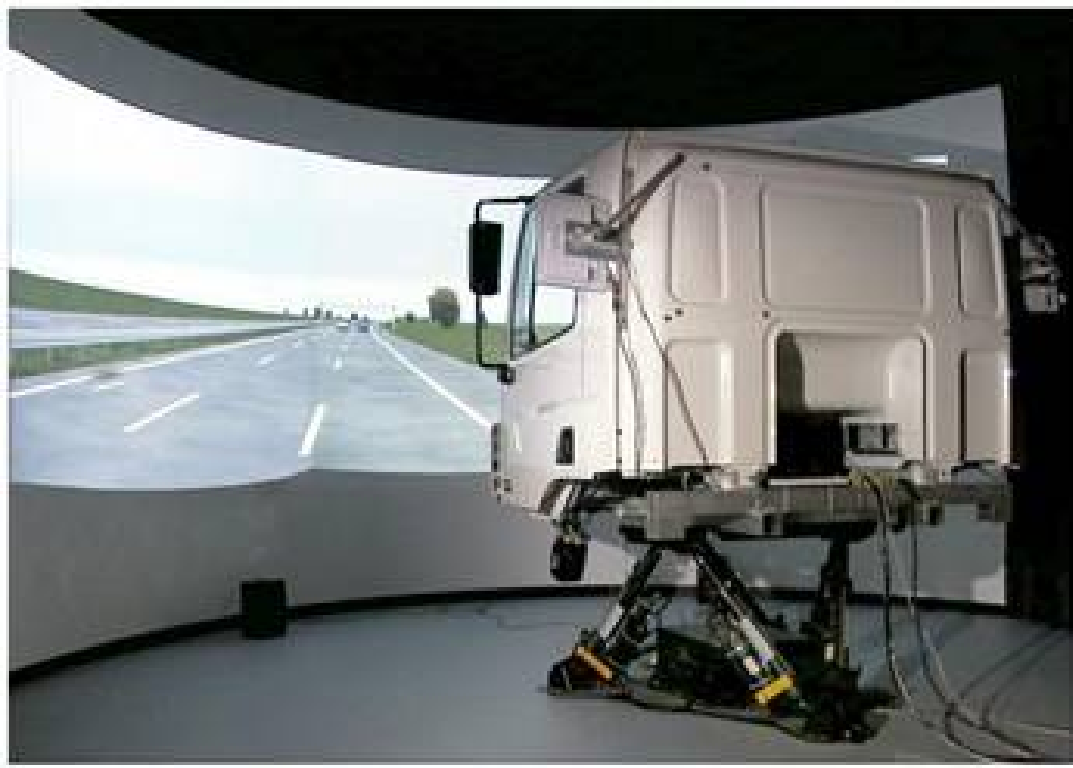
Figure 5. Type D simulator: dynamic driving simulator.
