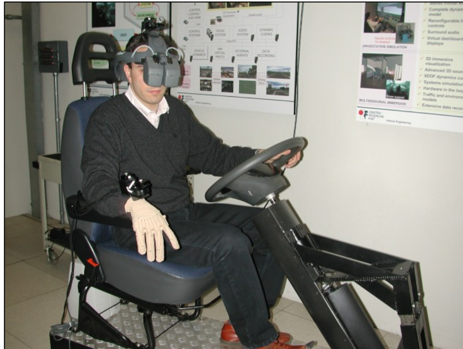
Figure 7. Type F simulator: Head-Mounted-Device (HMD) simulator.
