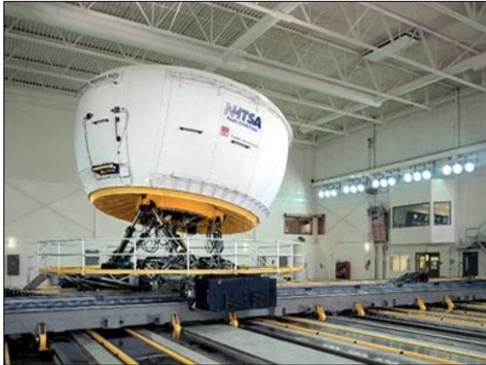
Figure 6. Type E simulator: advanced driving simulator.
