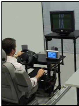
Fig. 1: Example of entry-level system (low-level fidelity system).
